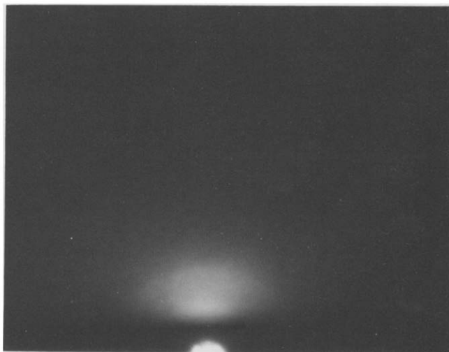
Figure 3 Electron diffraction pattern obtained from a decyltrichlorosilane film adsorbed onto aluminium mirrors
