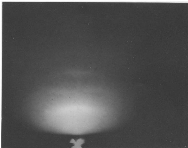
Figure 4 Electron diffraction pattern obtained from an octadecyltrichlorosilane film adsorbed onto aluminium mirrors
